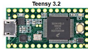
Teensy 3.2 72 MHz Cortex-M4 3.3V signals, 5V tolerant
