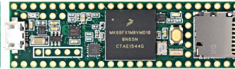
Teensy 3.5 120 MHz Cortex-M4F 3.3V signals, 5V tolerant
