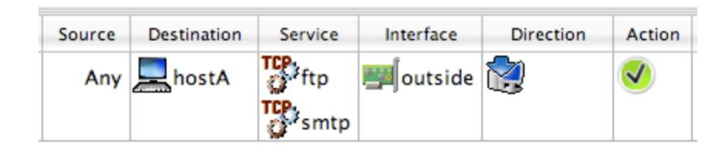
pass in quick on en0 inet proto tcp \
